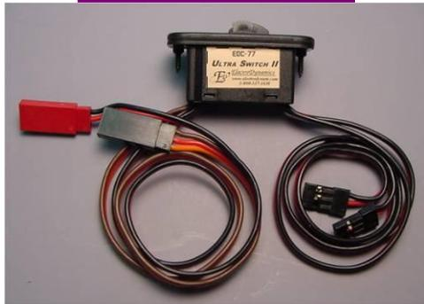
Heavy-Duty, 8A max. Ultra Switch II designed specifically to match the ED-Nano 2S1P Rx battery for *No-Hassle, Plug-and-Play* use
