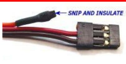
**Using an ED-Nano (A123) battery in an existing model already equipped with a 3-wire Switch**
