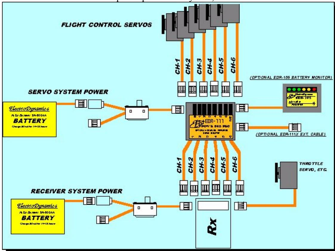
Larger control loads = heating effect on Receiver power bus.
