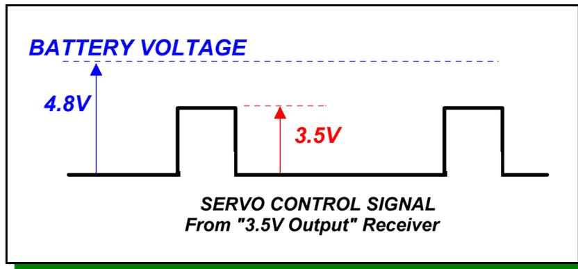
Most RC servos will operate fine with a 3.5V control signal, but some will become intermittent if the signal falls much below this.
