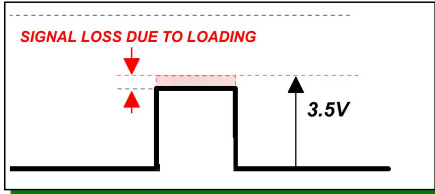
Some servos utilize circuits that set an input threshold level at a certain fraction of the power line voltage, so that any signal below the threshold will be rejected as random noise.
