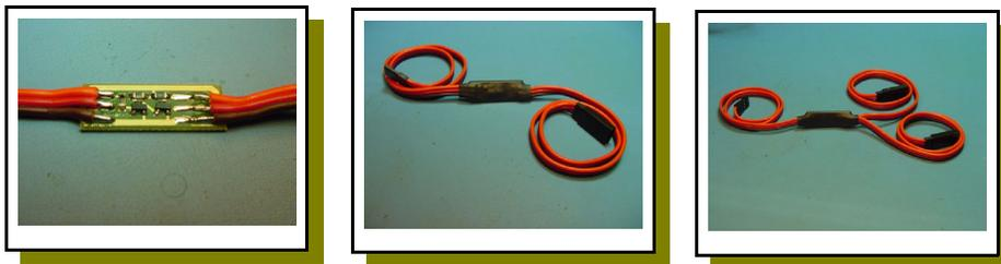
The rule of thumb with Buffer Amplifiers is: “avoid cable runs with more than 24” of unbuffered cable”. I.e., for a 36” run, use one buffer in the middle at 18”; for a 60” run, use two buffers, at the 20” point and the 40” point.
