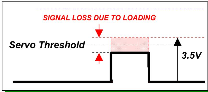
***Solution?*** Inline Buffer Amplifiers (our EDR-1040) or buffered extension leads amplify the receiver signal from below 2V to the full power supply voltage.
