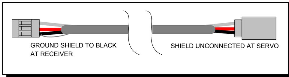
And, an improperly terminated/grounded shielded cable can make matters worse, actually acting as an antenna amplifier, feeding RF into the extension!
